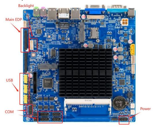
The location of the plug is detailed in the figure below
