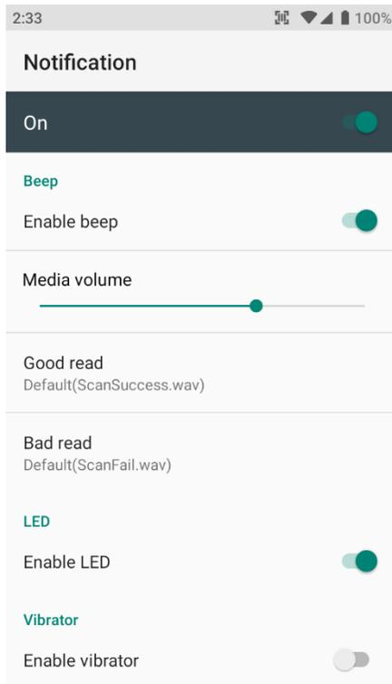
In the **Notification**, you can change the volume level, notification sound, LED and vibration option
