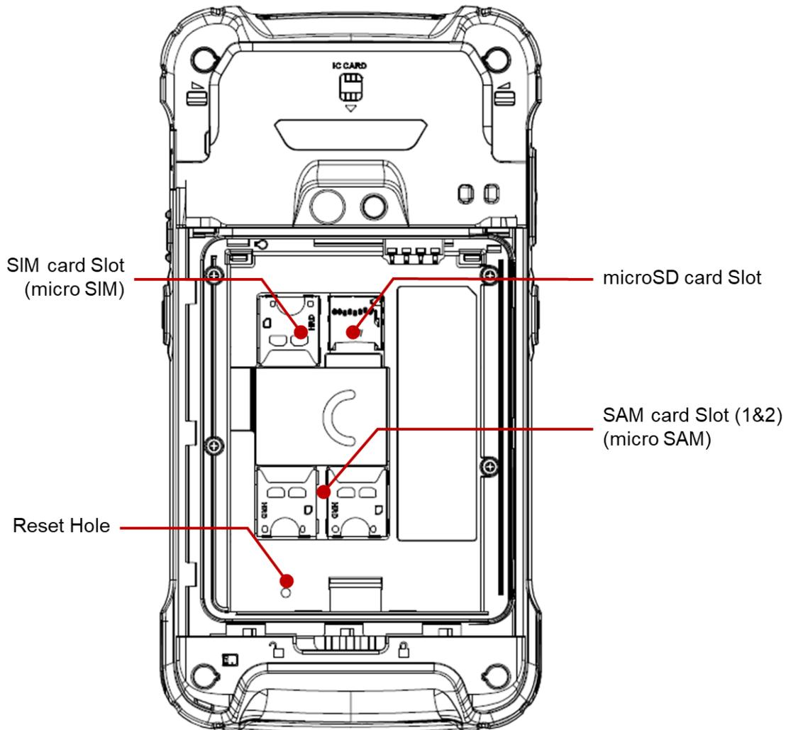
**Note 1:** PM90 only supports the micro SIM cards. Do not insert a size modified card with SIM adapter. Size modified card is thicker than the standard Nano SIM card and may damage the card slot
