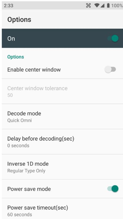
In the **Options**, you can enable/disable the **Center Window**, set **Decode mode**, **Power save mode** and enable/disable **Aimer & Illumination** option
