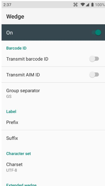
In the **Wedge**, you can enable/disable **Barcode ID** and **Aim ID**, set **Group separator**, **Prefix & Suffix**, **Character set** and **Extended Wedge**.
