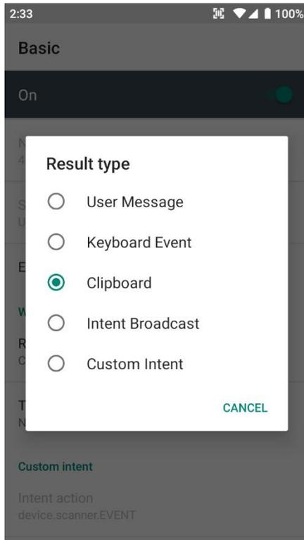
In the **Wedge menu** you can change, decode scan data's result type handling **User Message**, **Keyboard Event**, **Clipboard**, **Intent Broadcast** or **Custom Intent**
