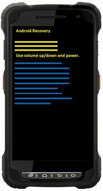
PM80 enter to the "Android Recovery" mode. In this mode, "Volume up" is "Move Up" in the menu tree and "Volume down" is "Move Down" in the menu tree. "Power Button" is "Select"
